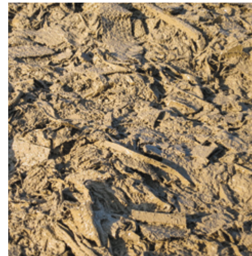
Posi-Shell Intermediate Cover directly on waste
